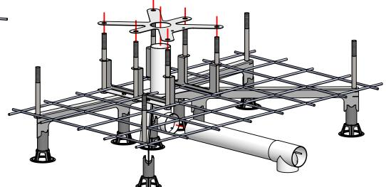
Slide the upper alignment plate onto the PVC pipe and down onto the six M20 bolts until it sits on the risers. Insert the horizontal PVC pipe into the PVC elbow with the "T" piece facing downwards, it is recommended to glue these together.
