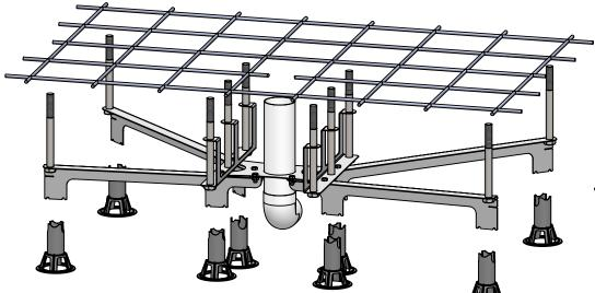
Place the frame on top of the concrete chairs making sure that the frame sits in the lowest part of the chairs. Place reinforcining mesh (must be SE92 reinforcing mesh or equivalent which is not included) on top of the kit set frame.
