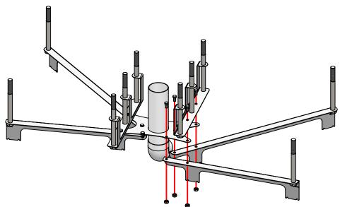
Bolt the legs and pole mounting bolts to the centre plate. The shorter legs go at the front and the longer legs go at the back of the block.
