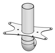
Slide the shorter PVC pipe through the centre plate with the elbow at the bottom.
