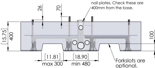
Centre the frame within the boxing and push the frame until the PVC pipe and the back nail plates are up against the boxing. Nail through the nail plates and into the boxing to hold the PVC pipe in place.
