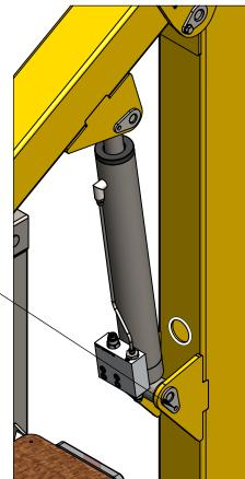
Fit the upper hydraulic ram with the appropriate ram pins, the pins are held in place by split pins.
