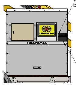
If a printer is included, plug in the printer power and data cables which are connected in the back of the computer console.
